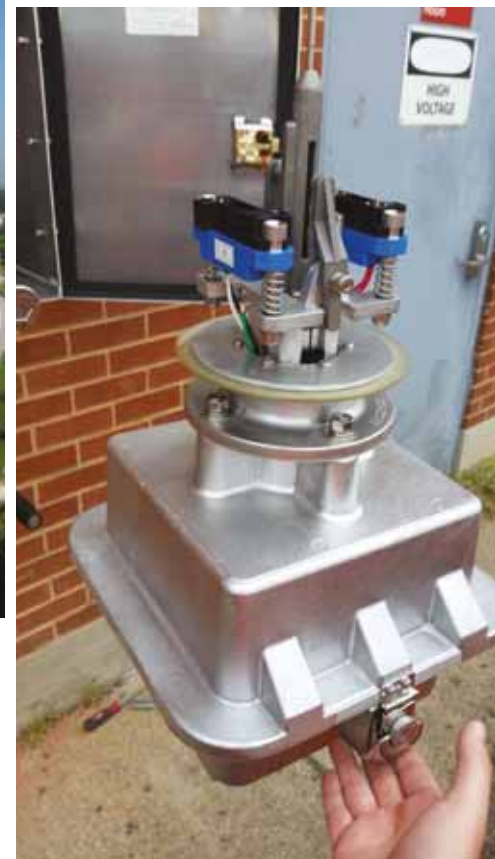
Gold plated pin and socket contacts with stainless steel alignment pins.
